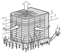
crowding the unit cause the outdoor unit to work harder and use more energy. Keep shrubbery trimmed away from the unit and periodically check for debris which may have collected around the unit.
